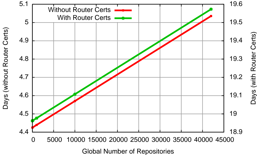
Figure 1: Between 4.3 and 5 days to sync (19 to 20 with router certs). That means that operators have to count on 9 to 10 days (or 38 to 40 with router certs) after making a change that they want RPs to pick up (twice the polling period).
